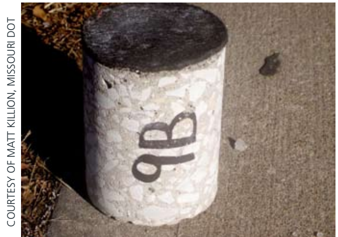
Figure 12. Core of Route D project showing overlay bonded to geotextile interlayer (underlying pavement not bonded, so core cannot be extracted).
