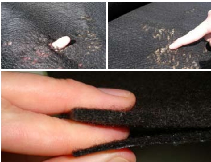
Figure 3. Undesirable thinness and partial melting of isolated areas of the Geotex 1201 compared to a thicker geotextile known to fully comply with German specifications.
